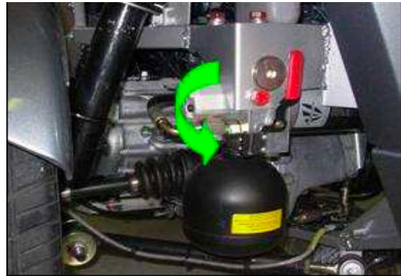
Turn the maintenance handle down and tilt the car fully over to the right, observing the eyeglass as the car tilts over.
