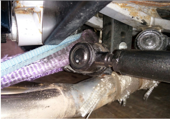
BACK - strap around the frame at the rear (where it is a V shape) and over the top of the pivot bar (do NOT strap around the track rods)
