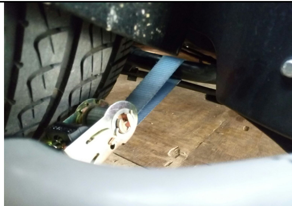
SIDES - strap around the anti-roll bar, to exit forward of the rear wheel and under the bullbar
