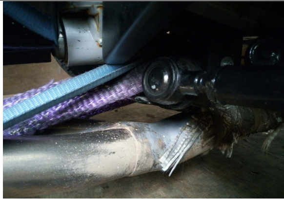
BACK - strap around the frame at the rear (where it is a V shape) and over the top of the pivot bar (do NOT strap around the track rods)
